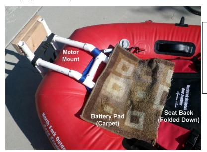
To avoid having a corner of the battery (or battery box) causing damage to the uncovered seat cushion you should put some kind of pad under the battery. I used a piece of discarded carpet.
