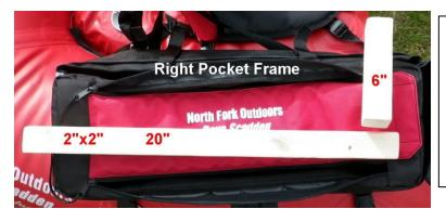
There are only two wood pieces for the utility rack inner wooden frame. The short piece is at the front, for attaching the right front deck. The utility rack will attach to the longer side piece.
