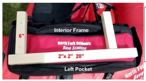
These are the wood pieces that will make the left pocket base for the rod holders and sonar. There will be a 3" pocket at the rear for holding the separate sonar battery.
