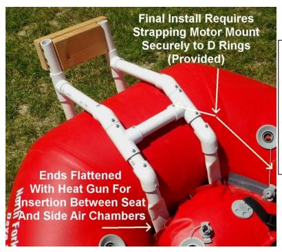
This picture shows how the motor mount has flattened bottom pieces to slide in the tight space between the main air chambers and the seat bottom. When all chambers are properly inflated...and straps connect the mount to the D-Rings...this motor mount is rock solid.
