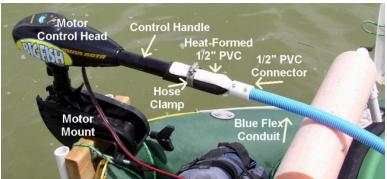
This is my "Smurf tube" motor extension handle. It is strong enough to run the motor but light and flexible. A full 8' long piece is usually less than \$3 in the electrical section of Lowes.
