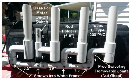
This is the modular rod rack on my Escape. The pocket is 21 inches long but I made the rod rack only 13" long...to keep the rods forward and easier to reach. Again, the rod tubes swing out for position adjustment and may be removed for more compact transport.
