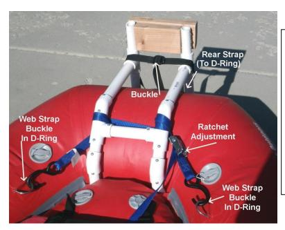
The PVC and wood motor mount fits snugly, but it requires straps to secure it against the motor pulling it out of position. Use strong and adjustable straps (blue ones) to hook the mount to the inner side D-rings as shown. The black straps go down to secure the bottom of the mount to the front bottom D-ring.
