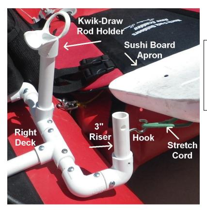
The rigid plastic apron is fitted with stretch cord. The loops on either side fit over either the PVC riser or the metal hook.
