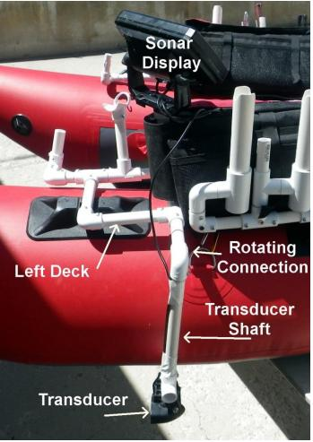
The transducer shaft freely rotates on the unglued connection. It moves down to the desirable 90 degree angle during fishing time. The more vertical the shaft the more accurate the sonar will read depths, bottom contours and fish targets.
