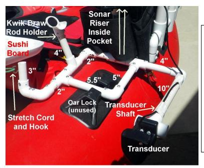
This is the left side front deck. It is a "multi-tasker". It holds a riser for the sonar display, the horizontal shaft for the sonar transducer, a riser to attach the left side of the rigid apron and a "kwik-draw" rod holder. It is secured to the wood frame inside the pocket by 3 long screws. It is held more securely by fitting the front crosspiece down inside the unused oar lock.
