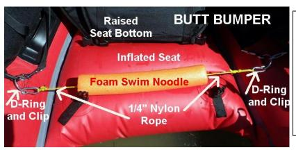
After a couple of trips in which the seat lost air pressure and let me slide forward I created a partial remedy by installing a "butt bumper". This was a length of foam swim noodle with a piece of 1/2" PVC in the middle.
