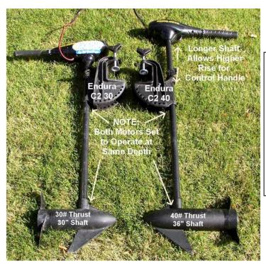
This picture shows a side by side comparison of the 30# and 40# motors. The 40 has a longer shaft which allows for running the motor deeper under your craft...or bringing the control head higher for easier reach.
