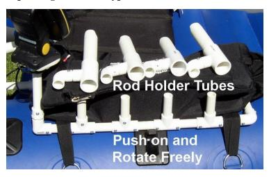
For a modular system, you make the PVC base first...then the rod tubes. The rod tubes swivel freely to adjust for position...and may be removed for more compact transport. This picture is of my old Renegade...with the rod rack held in place by the strap-down pockets.
